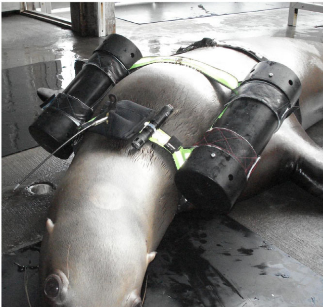
Fig. 1. A Steller sea lion equipped with a harness containing a pair of side-mounted PVC tubes, a very high frequency transmitter with an antenna between the tubes, and a cylindrical accelerometer next to the transmitter.
