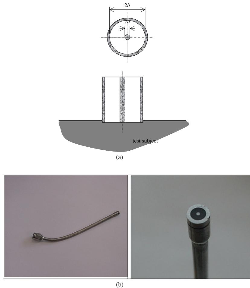
**Figure 1.** Dimensions and pictures of the probe used for the dielectric measurements. (a) Probe cross-section,  $a = 0.298$  mm and  $b = 2.5$  mm. (b) Photographs of the probe.
