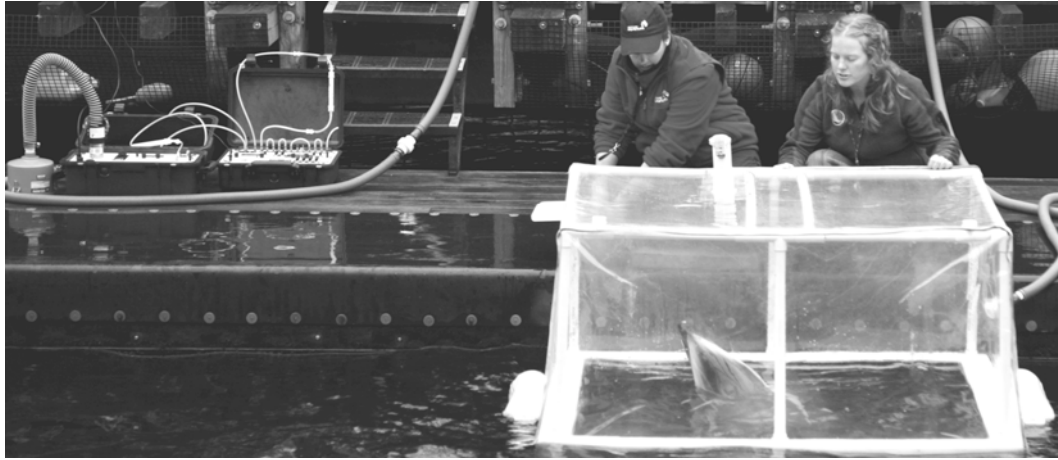
Figure 3.1 Experimental set up showing dolphin F001 stationed under the respiratory dome. The vacuum hose runs from the dome to the pump (far right to far left of photo) and ex-current air is sub-sampled in the Sable system (black boxes) where gas concentrations are determined.
