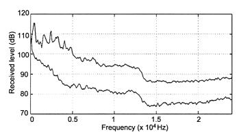
Fig. 4. Power spectral density comparing relative received noise level 100m from the experimental boat under fast (upper line) and slow (lower line) operating speeds.
