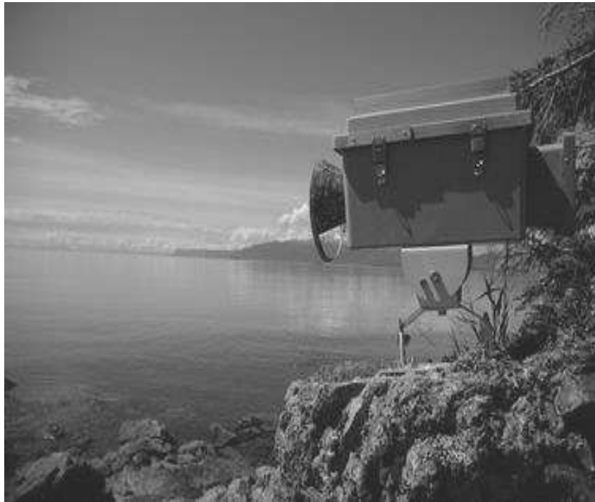
Figure 4.1. Outside view of the automated time-lapse camera system on Southwest Brothers Island.
