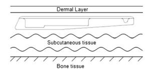
Fig. 3 In-service placement of implanted enclosure
