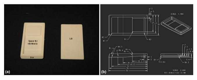
Fig. 1 (a) Photograph of alumina enclosure and (b) dimensions of alumina enclosure
