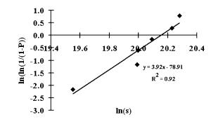
Fig. 4 Weibull diagram for compression tests
