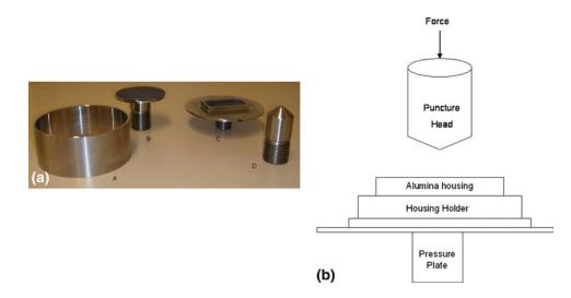
Fig. 2 (a) Test apparatus—A: shield, B: pressure plate, C: enclosure holder, D: puncture head and (b) application of loads using test apparatus during the puncture tests
