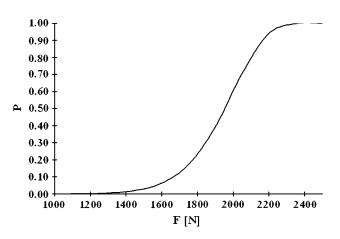
Fig. 7 Probability of failure of the enclosure vs. the applied puncture force
