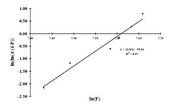
Fig. 6 Weibull diagram for puncture tests
